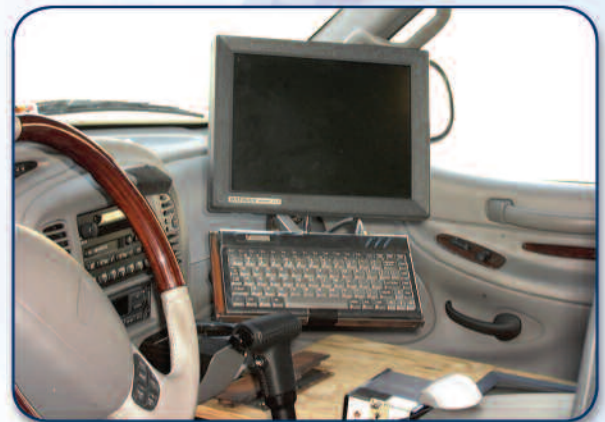
The In-Vehicle Data Acquisition System (IVDAS) was developed specifically to meet automotive proving ground test needs.
