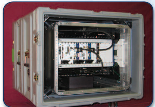
The RF Recorder (RFR) combines high-speed RF recording and playback capabilities to allow portable field recordings of RF signals up to 2.7 GHz for up to 6 hours.
